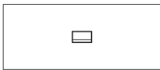
SAA grommet location Use with tops 30" - 40"d Specify VFA or VFD grommets separately
